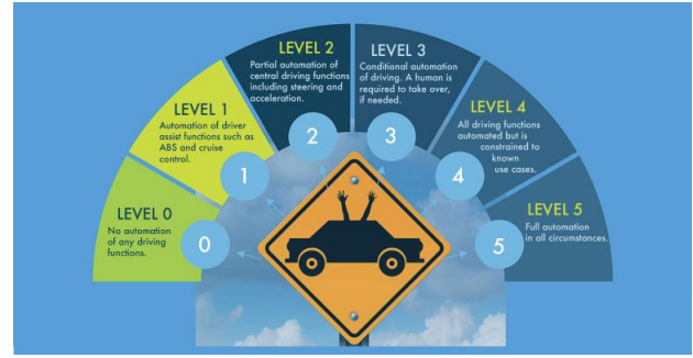
Fig. 1: Types of Autonomy levels in a Self-Driving car[1]
