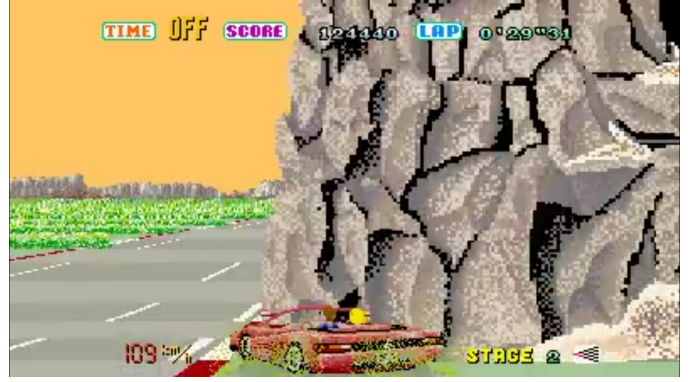
Fig. 7: A crash state on the simulator. The DDPG algorithm returns a penalty of -2.0 and resets the car during this state.
