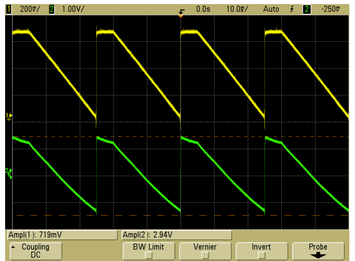
Fig. 10: Extron audio amplifier voltage waveform input (channel 1) and current output (channel 2), haptic feedback direction = left.
