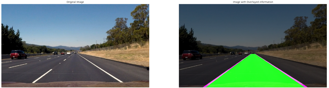
Figure 10: Overlaying polyfit lane lines and lane region-of-interest
